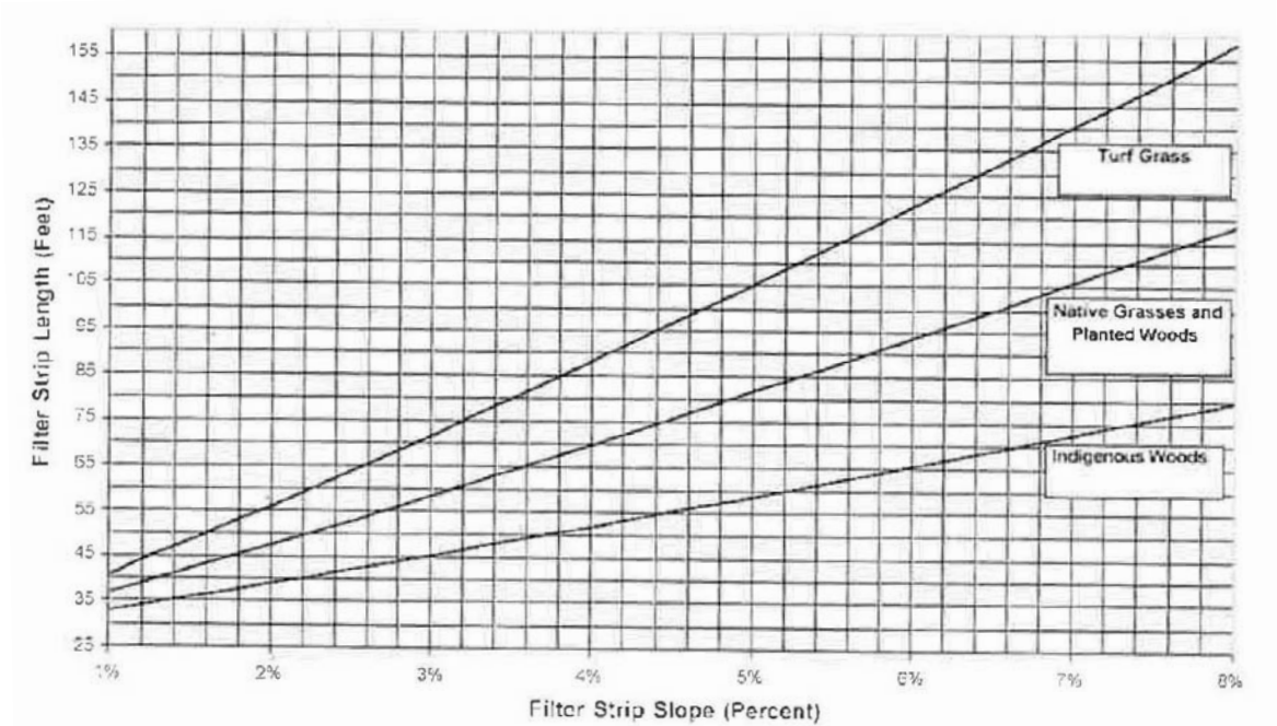
Figure 7d – Filter Strip Length (Clay Loam, Silty Clay, Clay soils with HSG D)
